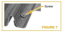
Screws: When self-drilling, self-tapping screws are used to connect the sidelaps of B-36-SS, W2-36-SS, W3-36-SS, N3-SS, N3-NS, or N-24-SS FORMLOK decks, they are to be minimum #10 x ¾ in. long. The "SS" designation indicates deck provided with modified female lip for screw fastening. See Figure 7. The "NS" designation for N3 FORMLOK deck indicates deck provided with nested sidelap. Deep and Shallow VERCOR decks have a nested sidelap.
