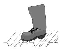
Button Punches: When sidelaps of FORMLOK decks are connected with button punches (BP), as shown in Figure 6, an average-sized person should be able to stand (not jump) on the flute adjacent to the attachment without the joint coming apart.
